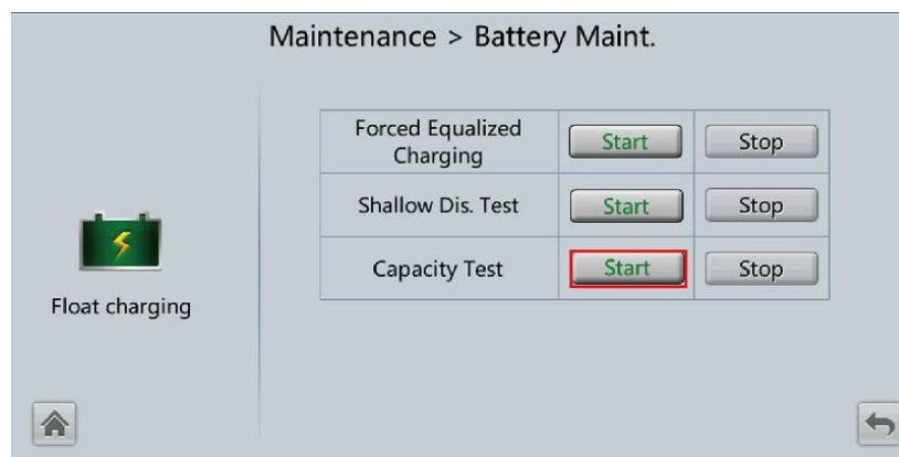
Figure 5-13 Starting a capacity test
