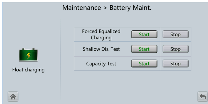
Figure 4-38 Battery Maint. (lead-acid battery)
