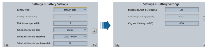
Figure 4-29 Battery settings (lithium battery)
